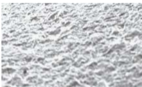
SEM Micrographs of machined surface (on the left) and sandblasted/acid-etched surface (on the right) (X221) – The sandblasted/acid-etched roughened surface of T.B.R. ® implants increases osseointegration capacity in comparison with machined surface.
