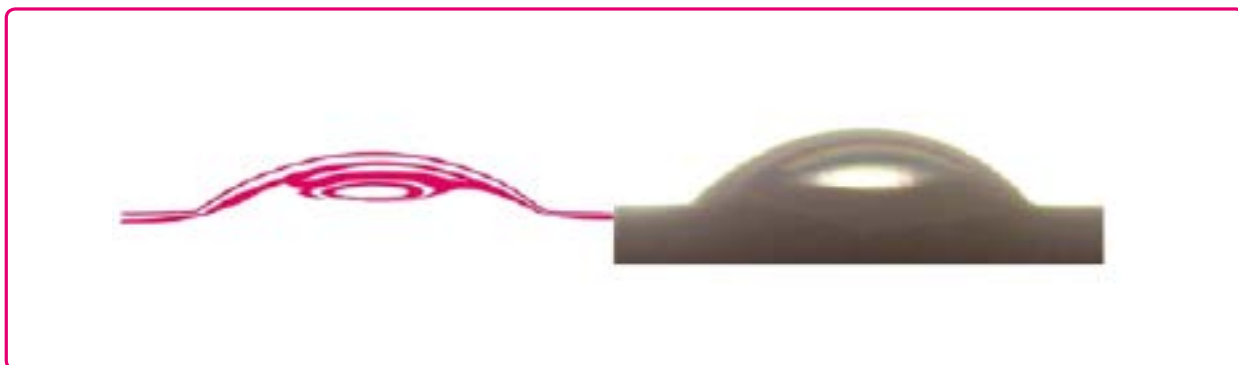
Figure 2. The angular value of zirconium abutment obtained by sessile water drop: 137.99°.
